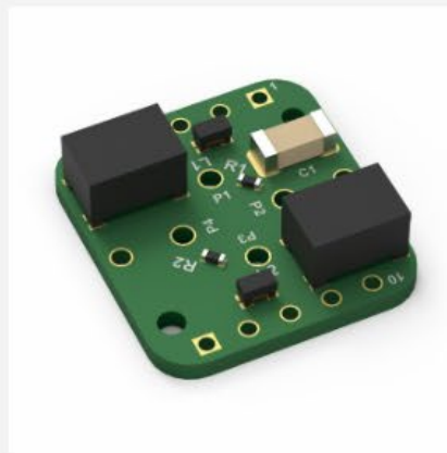
Integrated filter design for 10/100 Base-T Ethernet applications according to IEEE 802.3u
