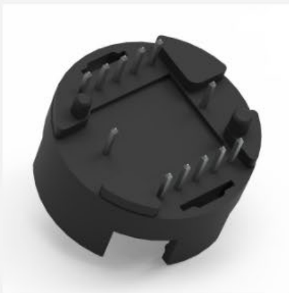
LCP bottom with THR pins and high spacers/standoff (1.4 mm) for optimum air circulation during soldering process
